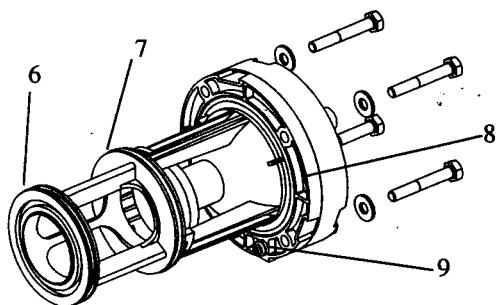
3 - No Hard Water Bypass Valve Cartridge
